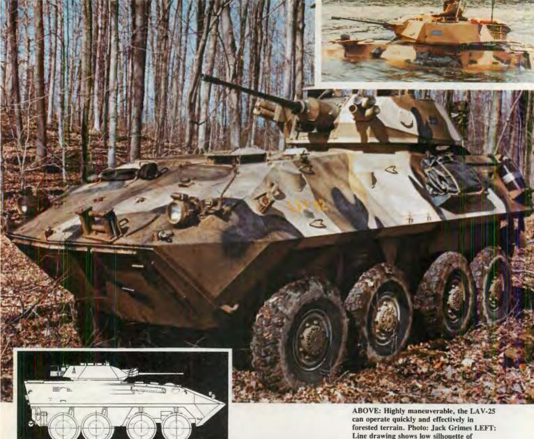
ABOVE: Highly maneuverable, the LAV-25 can operate quickly and effectively in forested terrain. Photo: Jack Grimes LEFT: Line drawing shows low silhouette of LAV-25. BELOW LEFT: Although this shallow pond will not test the swimming capabilities of the LAV, it has the ability to plunge through deep water by using its twin screws (see top photo). Photo: Jack Grimes
